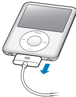
If your Dock connector is larger than the one shown, squeeze both sides of the connector while removing.
