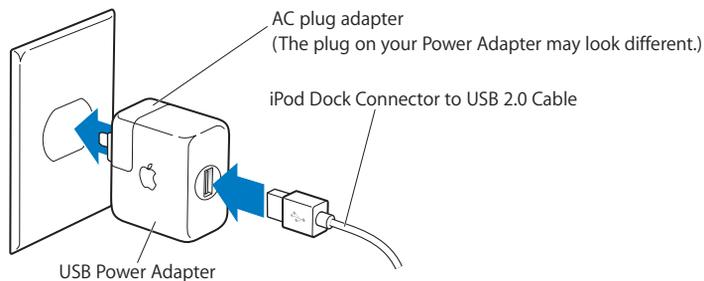
**WARNING:** Make sure the power adapter is fully assembled before plugging it into an electrical outlet.
